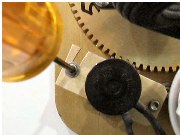
Step 12: Drive Polang to upper and lower electrical limits and verify drive direction & full range of motion of feed assembly.
