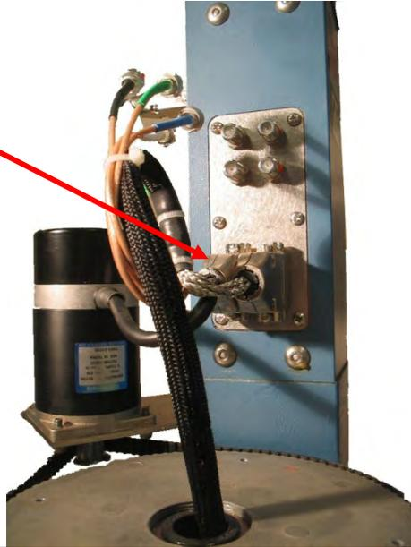
Using snips, cut the Tie Wrap holding AZ Motor Wire harness and Pedestal Interface Harness together.
