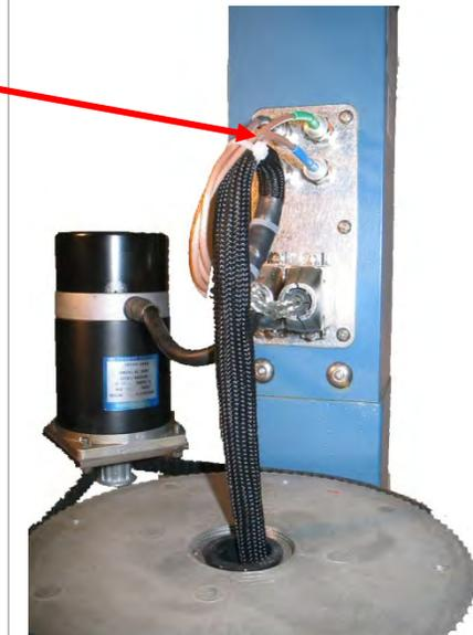
Using a 2mm Flat blade screwdriver loosen retaining screws securing both D-Sub connectors to AZ Post Connector Panel and remove.
