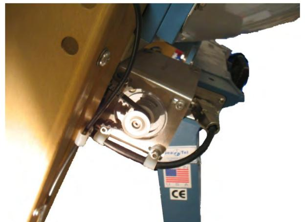
Rotate reflector from upper physical stop to lower physical stop and verify that the motor sprocket and the belt do not rub against elevation pan and that the belt runs inline with both sprockets. Incorrect belt travel is most frequently caused by incorrect sprocket placement on elevation motor shaft. Check and/or adjust antenna balance.
