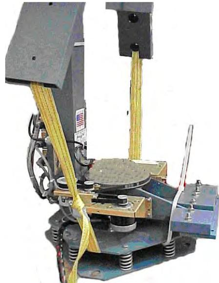
**CAUTION:** *Tighten the straps ONLY tight enough to restrain the antenna. When restrained the antenna will only be able to move about an inch in any direction. DO NOT OVER-TIGHTEN.*
