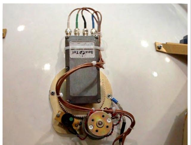
If you are replacing the LNB with the same style LNB, loosen the Allen set screws on the existing LNB mounting collar (three set screws, 120 degrees apart) and extract it from the mounting collar. If you are changing the LNB to a different style LNB, loosen the four screws that attach the mounting collar to the driven gear and remove the LNB and mounting collar.
