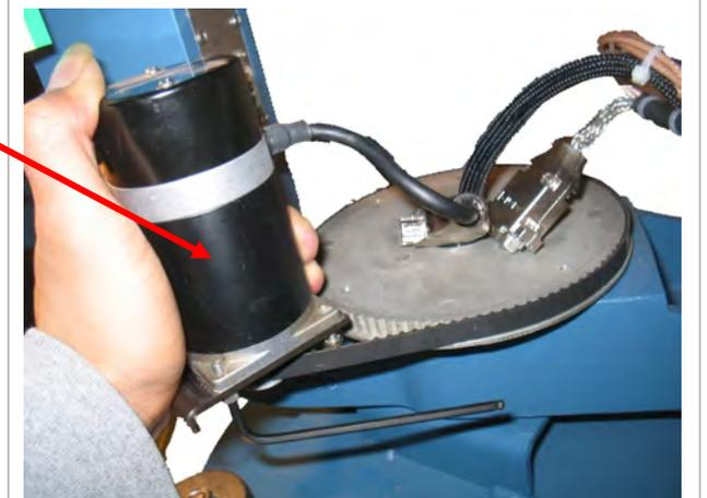
Rotate Antenna from CCW stop to CW stop while observing belt. Check to see the belt does not rub against motor mounting hardware and that the belt remains level with both sprockets.
