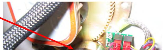
Disconnect Pol Pot IDC connector from motor termination PCB.
