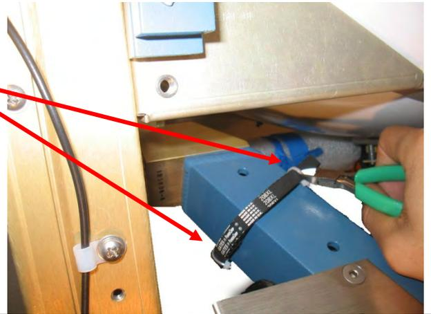
Install replacement belt around the elevation driven sprocket and elevation motor sprocket. Swivel the elevation motor bracket to CL beam (away from the reflector) and re-install the two screws removed in step 1. Using Loctite 222 tighten all four screws removed/loosened in step 1.
