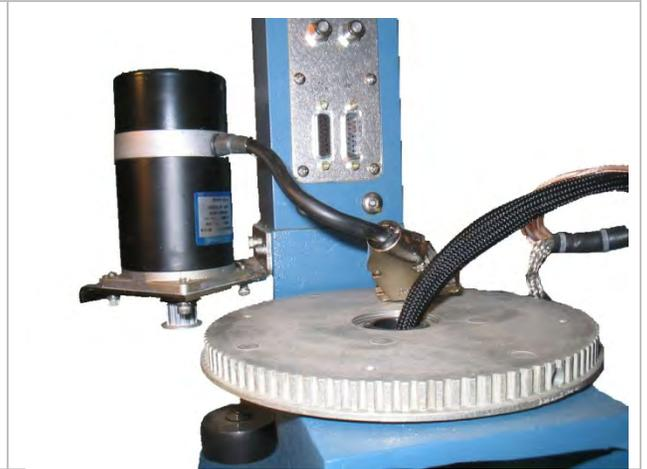
Place replacement belt around Azimuth motor sprocket, with interface harness and RF cables through the center of the belt. Place the belt don onto the teeth of the Azimuth driven sprocket.
