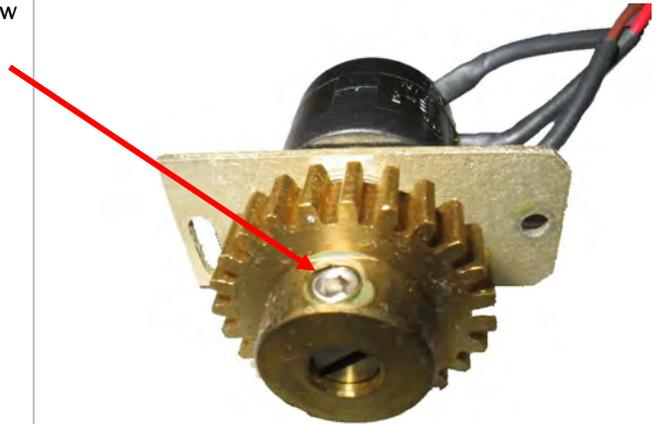
Using a 1/2" wrench remove nut and lock washer securing Pol Pot to bracket. Save all hardware for future use.
